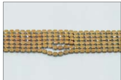
Too little solder
