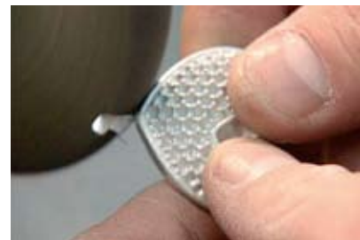
6 The cast model achieved by this process is ground and polished in preparation for the plating process.
