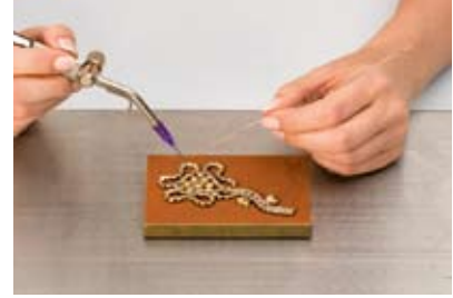
3 Solder the required spots.
