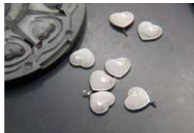
5 After cooling and removing from the mold, the casting channels are cut off.
