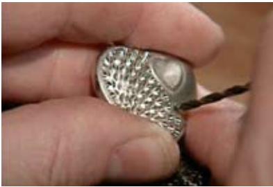
1 Several original models are shaped out of metal, which must already exhibit an excellent surface quality. The expected shrinkage during casting must be taken into account.
