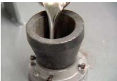
4 The completed rubber molds are filled with the molten metal alloy (centrifugal casting procedure).
