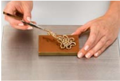
4 Remove the soldered Cupchain from the mold.
