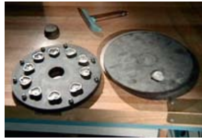
2 A rubber mold is vulcanized from these models and then a rubber casting model is made.
