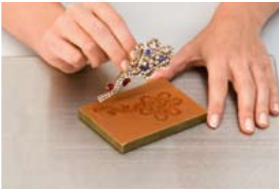
4 Once the material hardens, the original model can be removed
