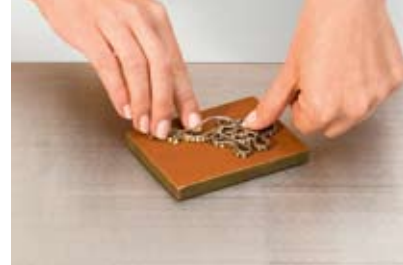
3 Pressing the original model into a suitable impression material
