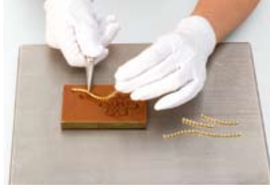
2 Put the Cupchain in the solder mold.
