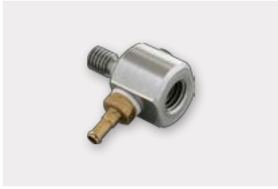
Vacuum adapter with M6 outer thread for fixing to the fly press and M8 inner thread to hold the upper die. Art. 9040/023
