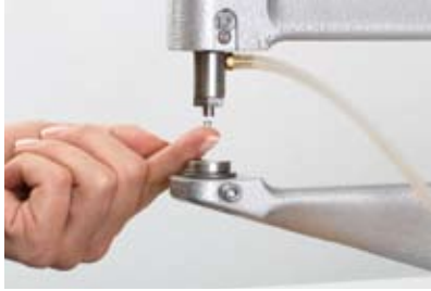
1 Place the Rose Pin in the upper die.
