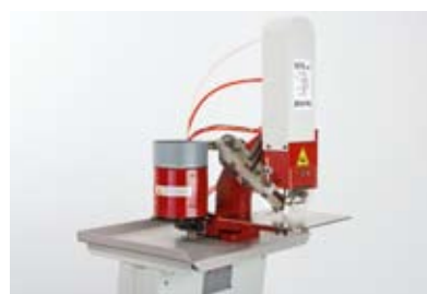
Some SWAROVSKI ELEMENTS can be applied using fully automatic attaching machines (e.g. Rose Pins). In this process, the feed on the machine must be adjusted to the element being processed.
