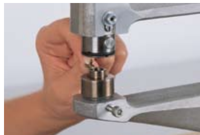
2 Place the arrow pin in the lower die.
