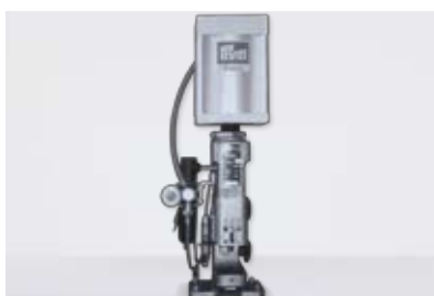
The pneumatic press enables quick application of crystal elements.
