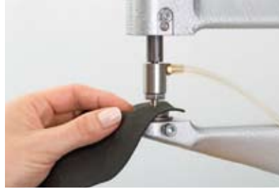
2 Position the carrier material and apply. Regulate the offset/pressure using the adjustable stop.
