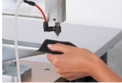
5 Position the carrier material and apply. Regulate the offset/pressure using the adjustable stop.
