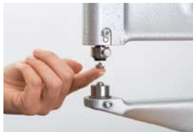
2 Place the ball part in the upper die.
