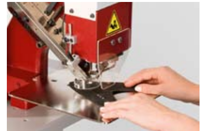
3 Position the carrier material and apply.
