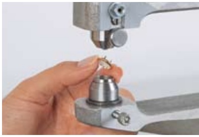
1 Place the Decorative Button/upper part of the Snap Fastener in the lower die, with the claws pointing upwards.
