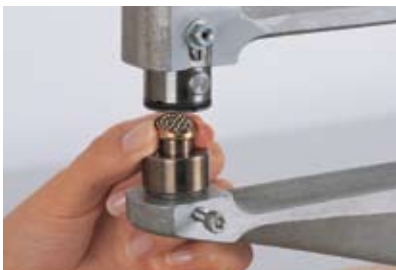
1 Place the top part of the Jeans Button in the upper die.
