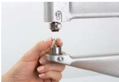
1 Place the pronged ring in the lower die, with the prongs pointing upwards.
