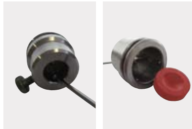
2 Use the changing pin to slowly slide the plastic insert out of the attaching die from above, through the hole.
