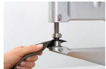
3 Apply the product to the textile in the previously marked position, ensuring it is on the right side of the fabric. Regulate the offset/pressure using the adjustable stop
