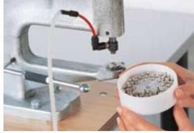
2 Gently shake the Rivets into the openings provided.
