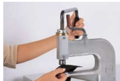
3 Carry out the application in the desired position. Regulate the offset/pressure using the adjustable stop.
