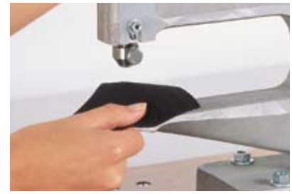
3 Apply the product to the textile in the previously marked position. Regulate the offset/pressure using the adjustable stop.
